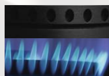
Oversized burner ports
